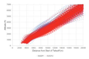
While the trial was conducted off the existing runway, the following diagram transfers the trial aircraft across to the new runway to show aircraft altitudes at distances from the point of take-off over residential areas. It also shows the two noise abatement departure procedures and the area of potential improvement the trial investigated.
