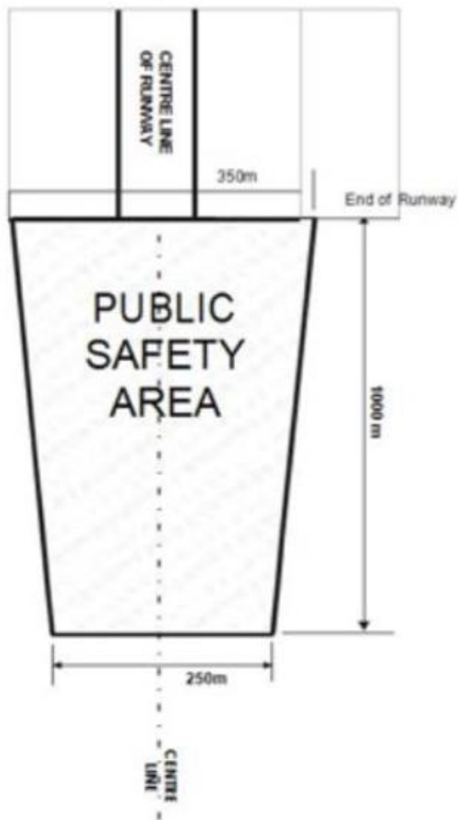
Figure 15 Queensland Public Safety Area
